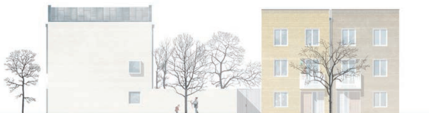
The tall parapets of the town houses of Eagle Foundry Street conceal a shallow pitched roof behind
